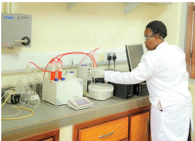
Picture 22: Grace Lajwe, Principal Chemist using the Auto-titrator for elemental analysis of minerals.
