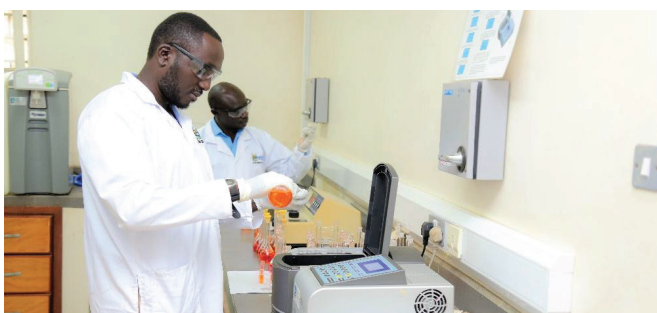
Picture 24: Henry Onyegbe, Senior Chemist using the Ultra Violet- Visible Spectrometer for qualitative and quantitative analysis of minerals, rocks and ore.
